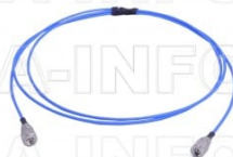
1.0M-1.0M-C010-3000 Flexible Cable Assembly 3000mm DC-110GHz 1.0mm Male to 1.0mm Male
